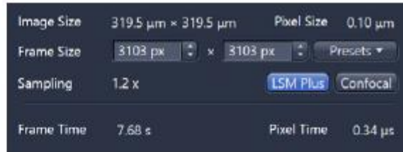
Figure 3 LSM Plus function with optimized acquisition settings. Sampling is set automatically and interlinked with the pinhole setting.
