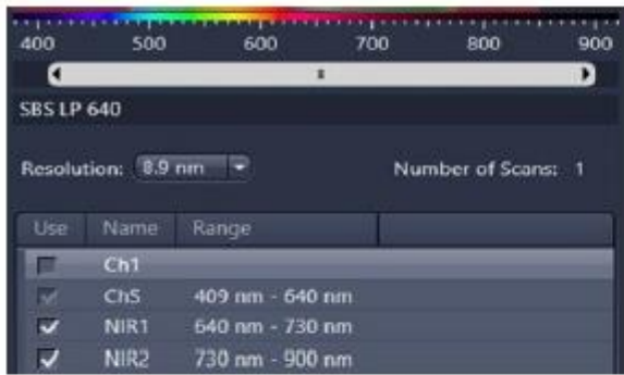
Figure 2 Spectral detection GUI, integrating several detector types which can be used with LSM Plus.
